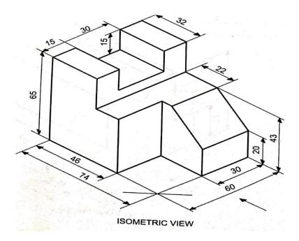
3. Draw to scale 1:1 the front view, top view and side view of the given machine block.
