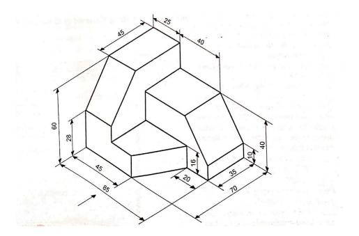
2. Draw to scale 1:1 the front view, top view and side view of the given machine block.
