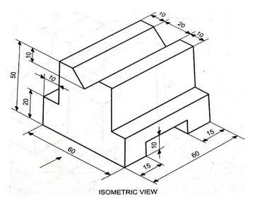
6. Draw to scale 1:1 the front view, top view and side view of the given machine block.
